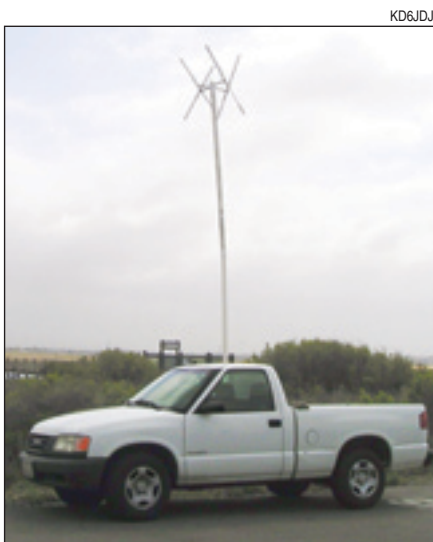
Figure 10 — Photograph of the Double Cross antenna mounted 2 \lambda above ground, at the beach in Southern California.
